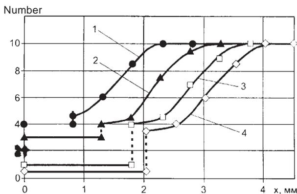
3 The dependence of the grain size on the distance from the weld axis: 1,2) Welding in helium, I<sub>w</sub> of 9 and 14 A, respectively; 3,4) Welding in argon, I<sub>w</sub> of 40 and 50 A, respectively.
