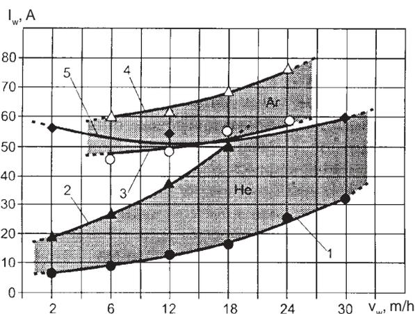
1 The range of permissible conditions of TIG welding in a shielding gas of resistance elements made of Kh23Yu5 alloy with a thickness of 0.8 mm.
