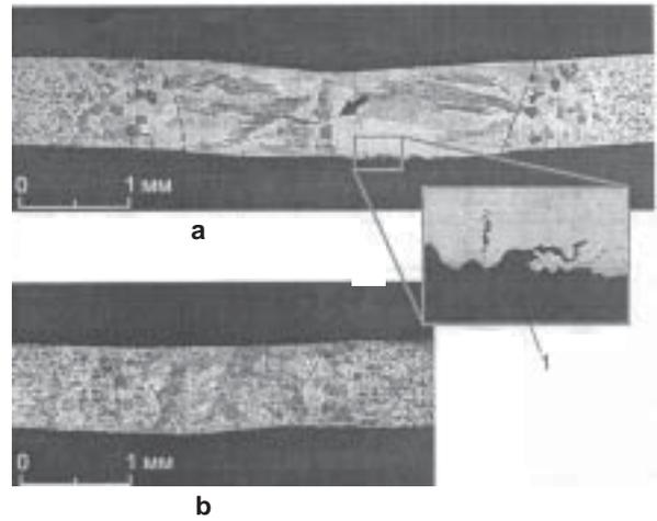
4 Structure (x25) of a welded joint reduced by argon- and helium-shielded arc welding.
