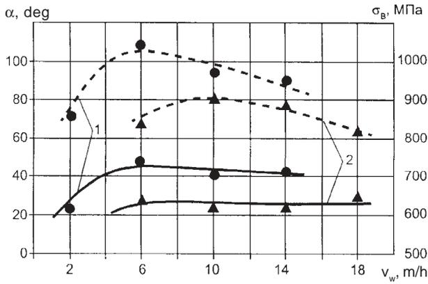
2 The dependence of the ultimate tensile strength (solid line) and the dent angle (broken line) of the welded joints on the conditions of helium-arc welding: 1,2) I of 14 and 22 A, respectively.
